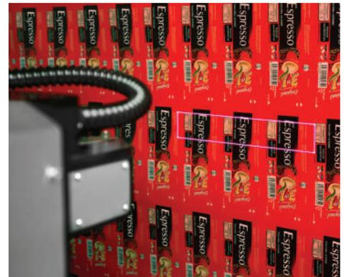
SLC350HD+ comes standard with aiming diode; expedites adjustments and cuts changeover time and waste
