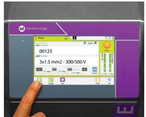
Extrusion-dedicated UI: metering, interleaving of 2 messages, quick access to counter setting, tolerance optimization, etc.
